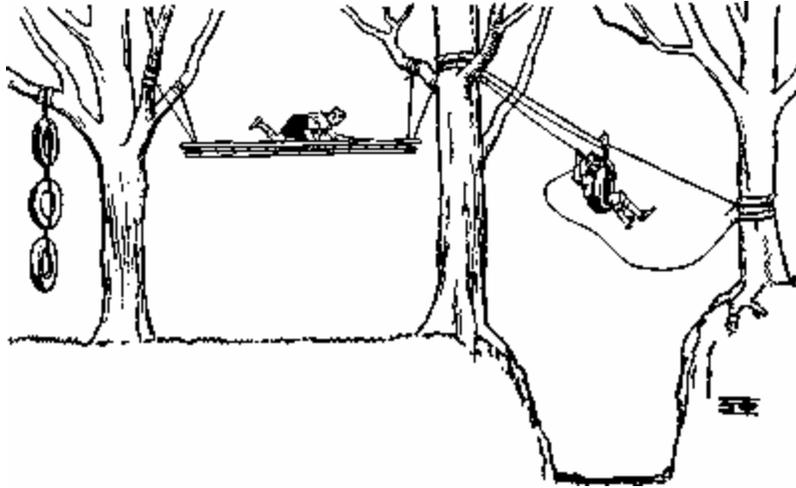
The third part is a self-controlled runway. Again, you will see, a tyre is used, this time in place of a bosun's chair. The great point about this apparatus is that it is workable from either end and the rider can control his rate of descent, which on a steep run is very important. When he has finished the next man can easily regain control of the seat and use it himself.
