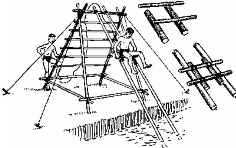
There is nothing technical in erecting an affair of this kind but I would remind you that the strain on the spars is considerable and they should therefore be of good quality, and the guys at the side need to be strong and very firmly anchored.
