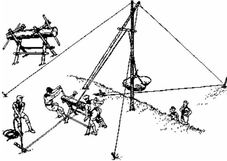
The artist has shown just one cross-tie to the sheer legs but I would recommend two and possibly three alongside each other, making a kind of laminated spar which will add enormously to the strength of the apparatus and consequently to its lifting capacity.
