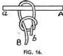
A form of the Sheet Bend, known as the Weaver's Knot, is used very largely in certain trades. It has the advantage of being very quickly tied, and of bringing the ends together so that they can be cut off with one snip, but it is not so suitable for use with a rope as the form already given, where the ends come off on different sides.
