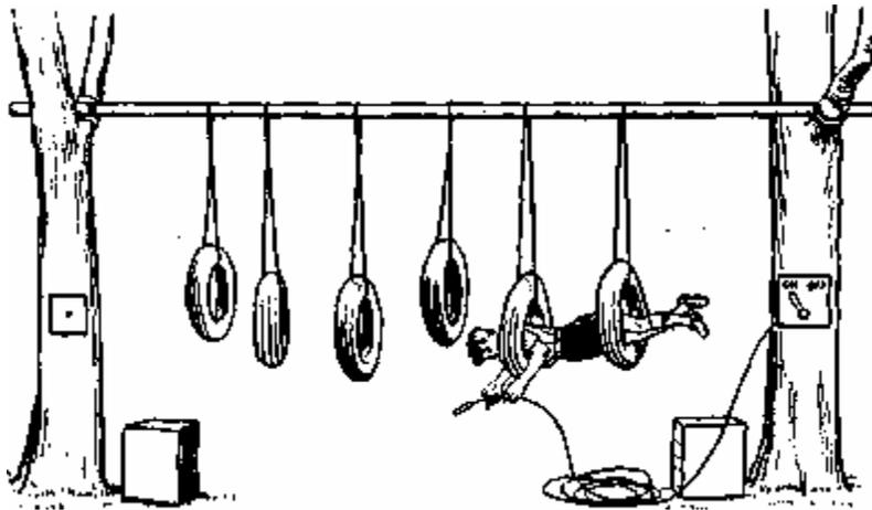
The construction is obvious. The supporting spar needs to be very solid and if you have any doubts about it, give it a pair of sheer legs as a centre support. The tyres must be hung at various heights, otherwise it becomes possible almost to dive through them, and remember that a tyre is heavy so it needs the support of a good piece of rope. Bicycle tyres will do for young Scouts but for Senior Scouts car tyres are a much better proposition and no more difficult to obtain.
