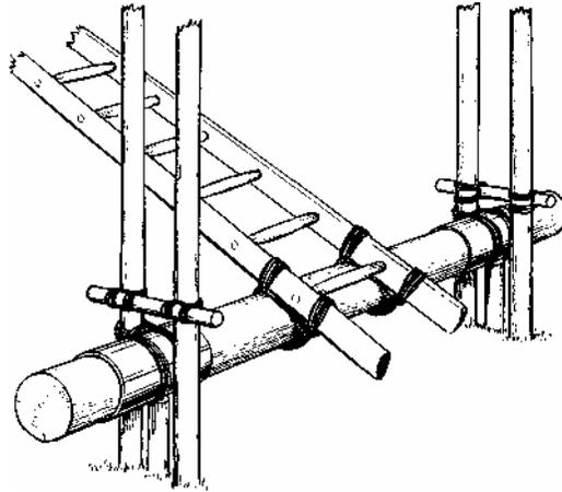
Note that the tin or the drum is lashed securely in position and is supported underneath so that it is the spar that is free to move inside the casing and not the casing itself.
