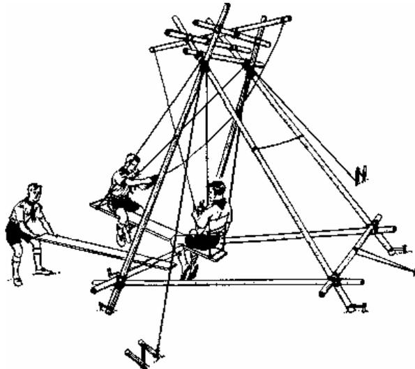
The braking device is not essential except that if you are using the apparatus as a money-making proposition you must have some method of stopping it otherwise an obstreperous customer can have a lot more than his money's worth. For use in a Scout camp the braking device can easily be dispensed with.
