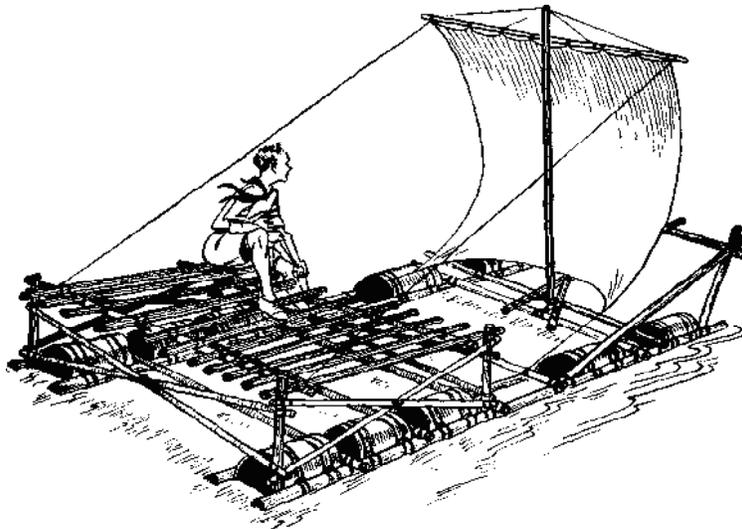
A word of warning: Don't let the deck be built too high above the drums. In any form of structure, the lower you can keep the centre of gravity the better, and if you have a very high
