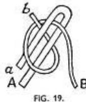
Tighten up knot by pulling on "standing part" of B.
