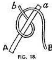
Pass the end of A over two turns of B and under one.
